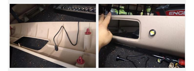
The light and switch runs off my second battery at the back. So I cut off the end off the 12V cable used for the LED strip originally to expose the positive and negative wires. The Eagle Eye wires were 4 strands of hair thick. My soldering skills are 0.1/10 as demonstrated below.
