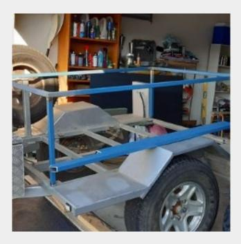
The frame structure is 30mm square tube with a 3mm sidewall. I wanted a trailer with a lid so I could access all the space.
